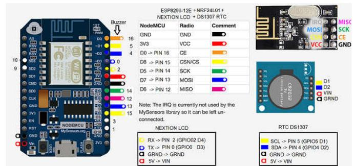
Figure 5 Conection Schemawith devices NodeMCU, Nextion, DS1307, NRF24L01+. Developed by the author
