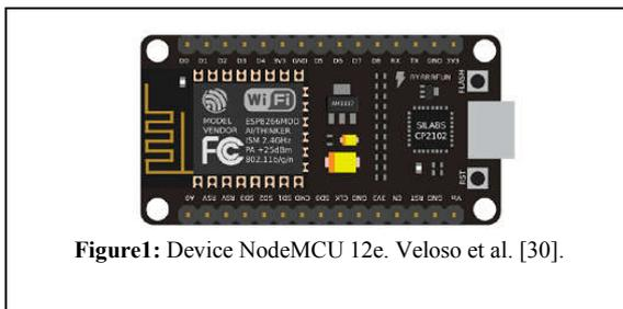
Figure1: Device NodeMCU 12e. Veloso et al. [30].
