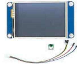
Figure 3 DeviceNextionNX3224T024. Itead[12].
