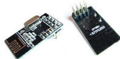
Figure 4 Device NRF24L01+. br-Arduino.org [3]
