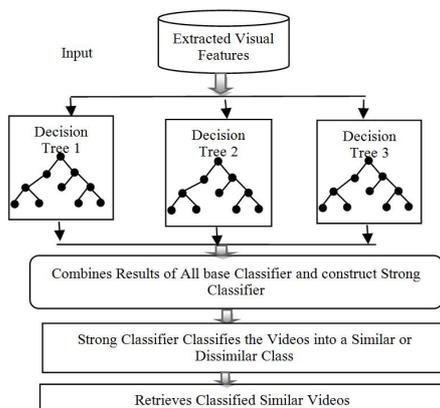
**Figure 3** Process of Gradient Boost Ensemble Classifier for Video Classification
