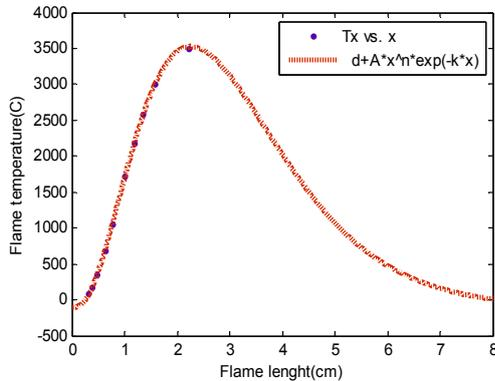
Figure 5 Flame temperature versus flame length of oxyacetylene flame (model II)
