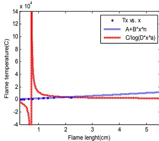
**Figure 4** Flame temperature versus flame length of oxyacetylene flame (model I)
